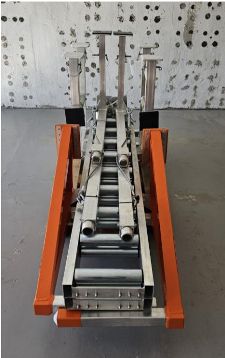
5: PUT CEILING SUPPORTS ON TOP
