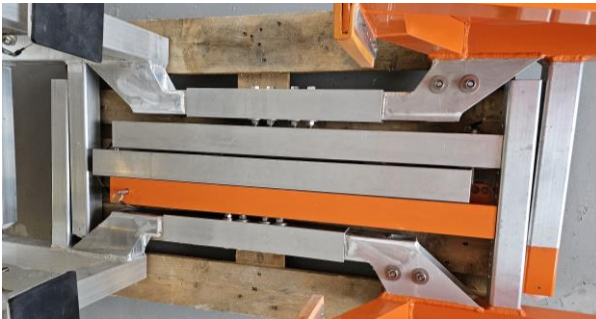
3: PUT ONE CENTRAL LATERAL BEAM BETWEEN THEM
