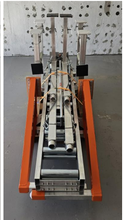
7: PUT THE PULLING HOOK ON TOP IN THE MIDDLE AND SECURE THE LOAD WITH RATCHET STRAPS
