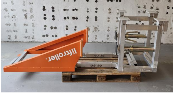
1: PUT BOTH SIDE FRAMES ON A PALLET.
