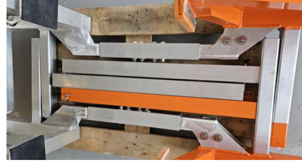
3: PUT ONE CENTRAL LATERAL BEAM BETWEEN THEM
